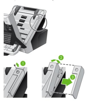
3. Gently pull the hardware integration pocket connector up and out of its recessed location.
